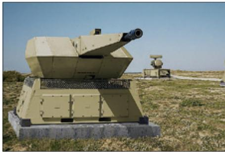
Modern Counter Rocket Artillery Mortar (C-RAM) systems can be readily adapted for the Counter PGM roles, but will require significantly better engagement radars, capable of tracking, sorting and engaging multiple inbound high speed PGMs. Depicted a Luftwaffe MANTIS/Skyshield 35 mm gun system, and a prototype high mobility Phalanx C-RAM system on a modified Oshkosh HEMMT chassis.
