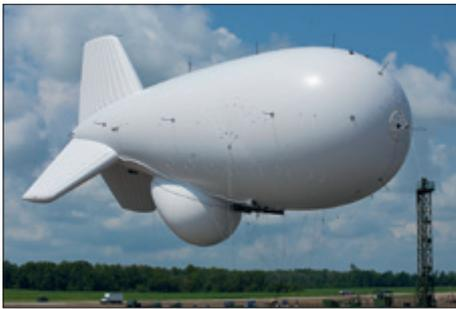
The JLENS aerostat based radar system was intended to provide over the horizon low altitude cruise missile engagement capability for the Patriot. It was cancelled in the latest round of United States defence cuts.
