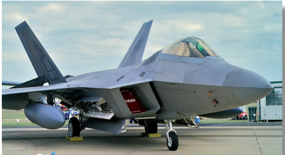
The Block 35 F-22A uses PAO liquid cooling for core mission avionics, and COTS processing hardware in several key systems.
