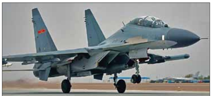
The KTRV/GNPP KAB-1500 with a subcalibre concrete piercing warhead will be available with two different laser seekers, an electro-optical seeker, and satellite guidance. Depicted a test drop and a PLAAF Flanker G, both with the precision electro-optical variant.
