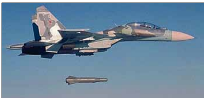
The KTRV/GNPP KAB-1500 with a subcalibre concrete piercing warhead will be available with two different laser seekers, an electro-optical seeker, and satellite guidance. Depicted a test drop and a PLAAF Flanker G, both with the precision electro-optical variant.
