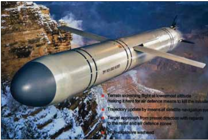
The land attack 3M14E Sizzler variant is a standard weapon for late model Kilo-class SSKs, which are widely used across Asia, and is intended for attacks on airfields. It is highly effective against revetted aircraft.
