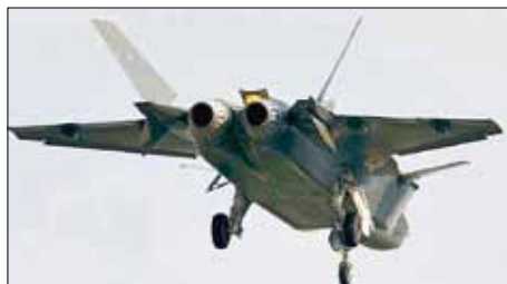
Aft view of the J-20. The axi-symmetric nozzles are the single greatest weakness of this otherwise robust stealth shaping design.
