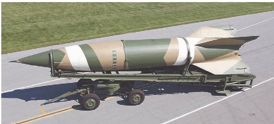
*A recently restored example of the A-4 on the Meillerwagen TEL, both owned by the US Air Force museum. Splinter camouflage was typical for operational weapons, using a range of patterns and colours.*
