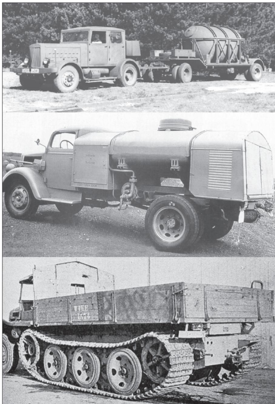
*Battery fuel train for the A-4, top to bottom: LOX tanker towed by Hanomag tractor, Opel Blitz S tanker truck, used for fuel and hydrogen peroxide supply, FAMO Sd.Kfz.9 18 tonne halftrack tow tractor used in difficult terrain.*
