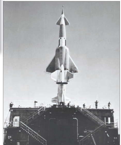
The cancelled N.A.A. Navaho was to be a 3,500 nautical mile intercontinental range nuclear armed Mach 3.5 ramjet GLCM.
