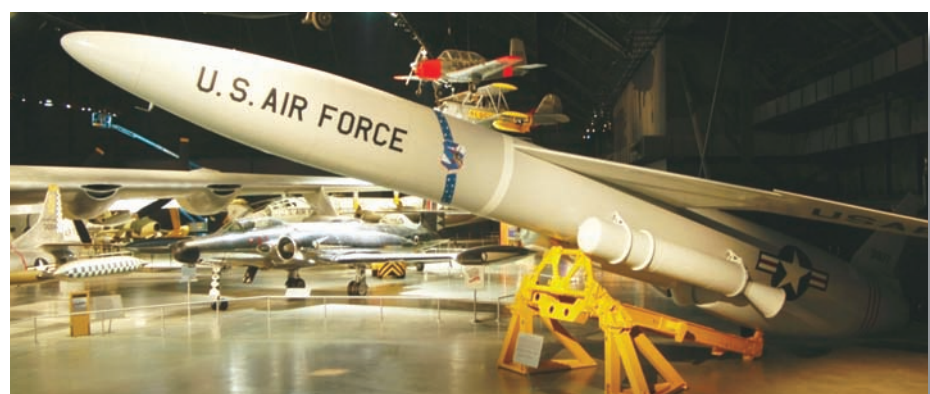
Northrop SM-62 Snark strategic cruise missile. This enormous 50,000 lb plus GLCM was built to directly attack the Soviet Union from US basing. It introduced the first stellar-inertial guidance system in a cruise missile.
