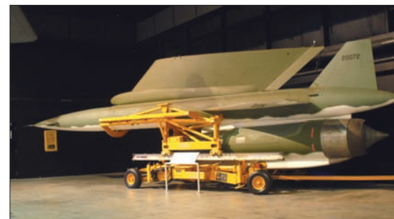
The N.A.A. AGM-28 Hound Dog was a supersonic 700 nautical mile range class cruise missile, carried operationally by the B-52 fleet until 1975. Over 700 were built. It used a liquid propellant booster stage for launch and climb to cruise altitude.
