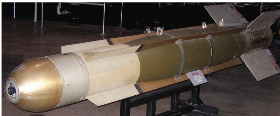
The Rockwell GBU-8/B 2,000 lb and GBU-9/B 3,000 lb HOBOS television guided bombs were used in the latter phase of the Vietnam war (Wikipedia).
