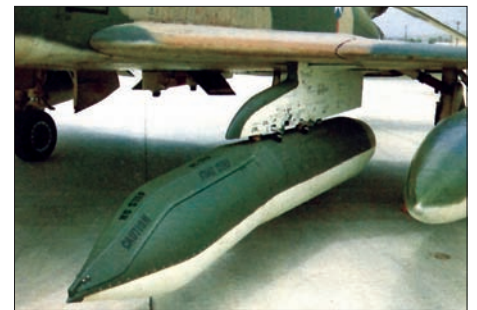
The Ford AVQ-10 Paveway laser targeting pod overcame the limitations of the earlier AVQ-9 Paveway Light cockpit designators and was the preferred system in 1972.
