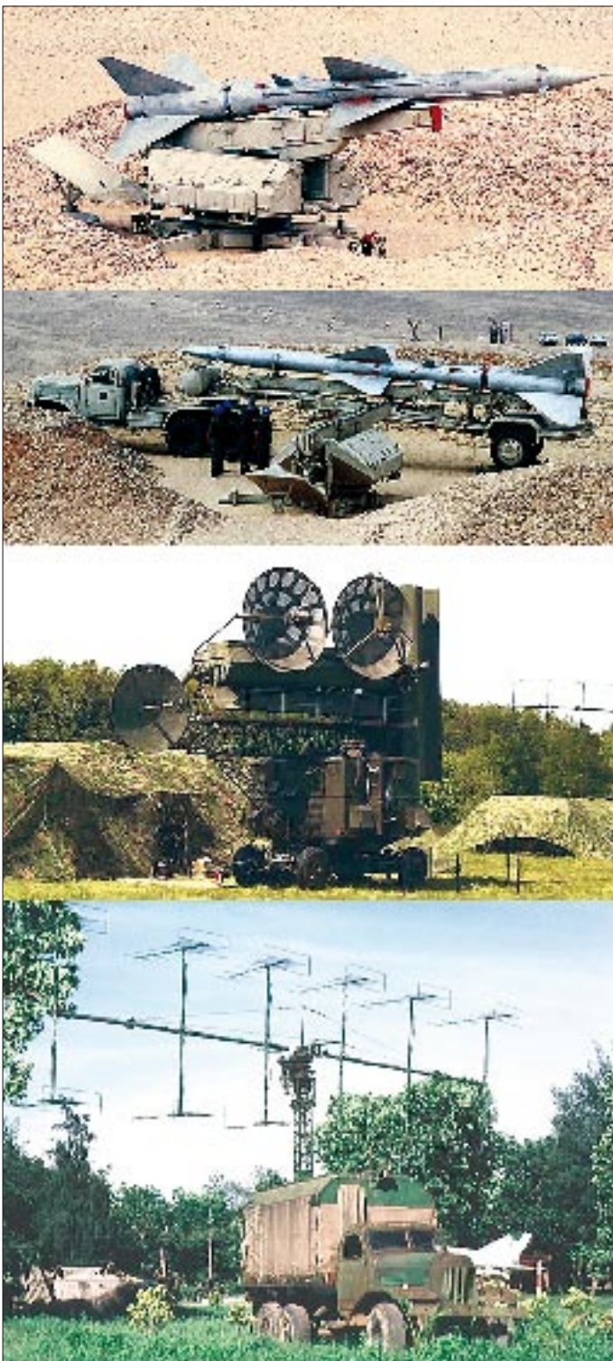
S-75 Dvina / SA-2 Guideline battery components top to bottom: V-750 missile round on SM-90 launcher, PR-11A transloader and SM-90, SNR-75 Fan Song radar, P-12 Spoon rest radar.
