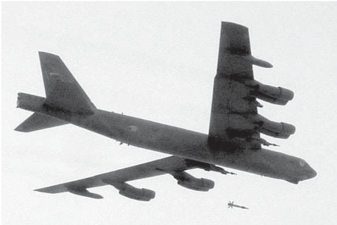
*This Boeing B-52H is the prototype system equipped with a Rafael Litening II laser targeting pod, which permits the B-52H to deliver laser guided weapons. The aircraft was reported to have engaged a pair of targets in the Tikrit area before the collapse of the Baathist regime. (US Air Force)*
