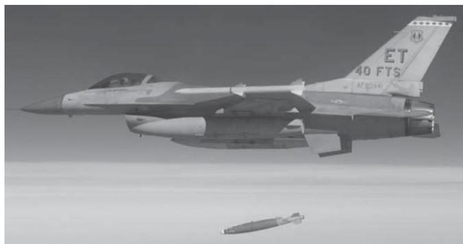
*The new Boeing GBU-38 500lb JDAM was first used enmasse during a B-2A strike, when a single aircraft disgorged no less than 80 rounds, each individually programmed to autonomously attack its own aimpoint (top). With a small Mk.82 warhead, the weapon is well suited to urban combat due to its smaller spalling and shrapnel footprint, compared to the standard Mk.84 2000lb GBU-31 (bottom). The weapon is planned for full scale production in 2004. (US Air Force)*
