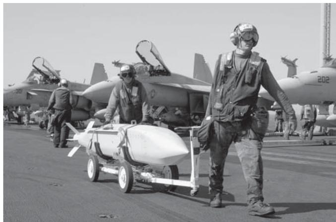
*The Raytheon AGM-154 Joint Stand Off Weapon is a US Navy led program, yielding a GPS aided inertially guided standoff glide weapon. Three basic variants were planned for – the AGM-154A carrying cluster bomblets, the AGM-154B carrying the BLU-108 SFW submunition and the AGM-154C with a terminal seeker and unitary warhead. To date the most frequently used model has been the AGM-154A – in effect a standoff accurate cluster weapon. (US Navy)*
