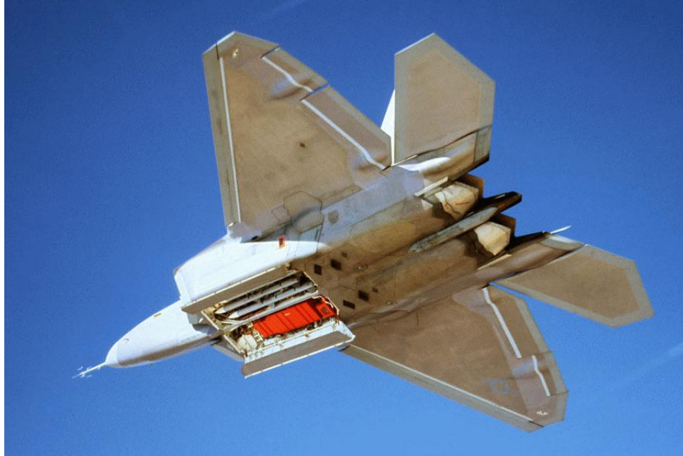
Figure 6: In terms of diversion range on internal fuel, total missile load and radar capability, the best candidate fighter to deal with a cruise missile threat is the F-22A, followed by a phased array equipped F-15E variant. The F-22A carries 6 AAMs internally and up to 8 on external pylons, the F-15 4 rounds on fuselage stations, 4 on inboard pylons and should provisioned for outboard pylons be fitted, an additional 4 rounds. The F-22A's APG-77 has by far the best detection range performance against small targets of any current fighter radar (USAF).
