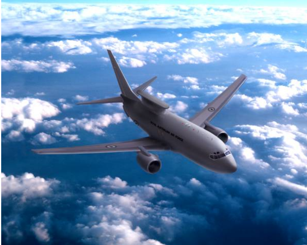
Figure 4: The Wedgetail program has been deferred and numerous reports from Canberra suggest that a cancellation may be imminent. The Wedgetail is based upon a Boeing 737-700/800 series airframe, equipped with a Northrop Grumman MESA phased array radar/IFF system, supplemented by an ESM receiver package and comprehensive communications suite. The MESA radar is widely acknowledged to have exceptional performance against small radar targets which makes it a particularly good choice for detecting and engaging cruise missiles.
