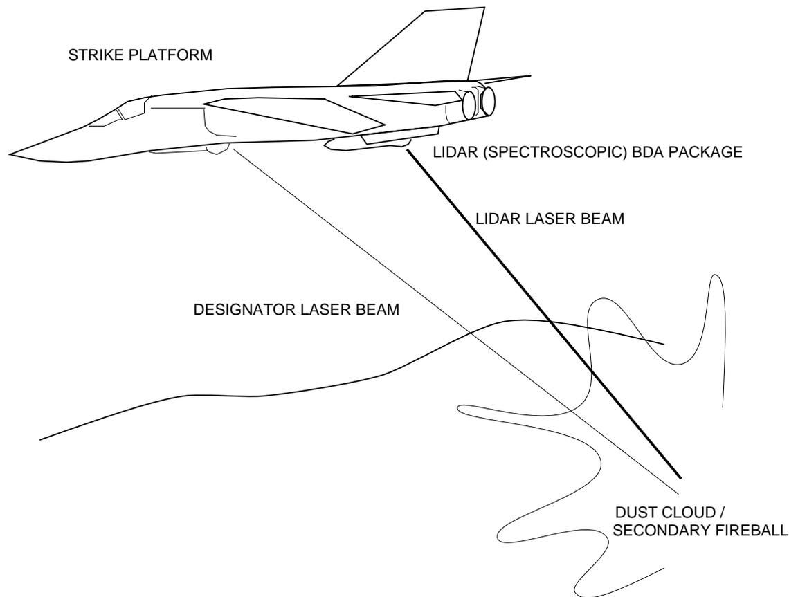
**FIG 1. LIDAR (OPTICAL ABSORPTION) SPECTROMETER USED AS BDA SENSOR**
