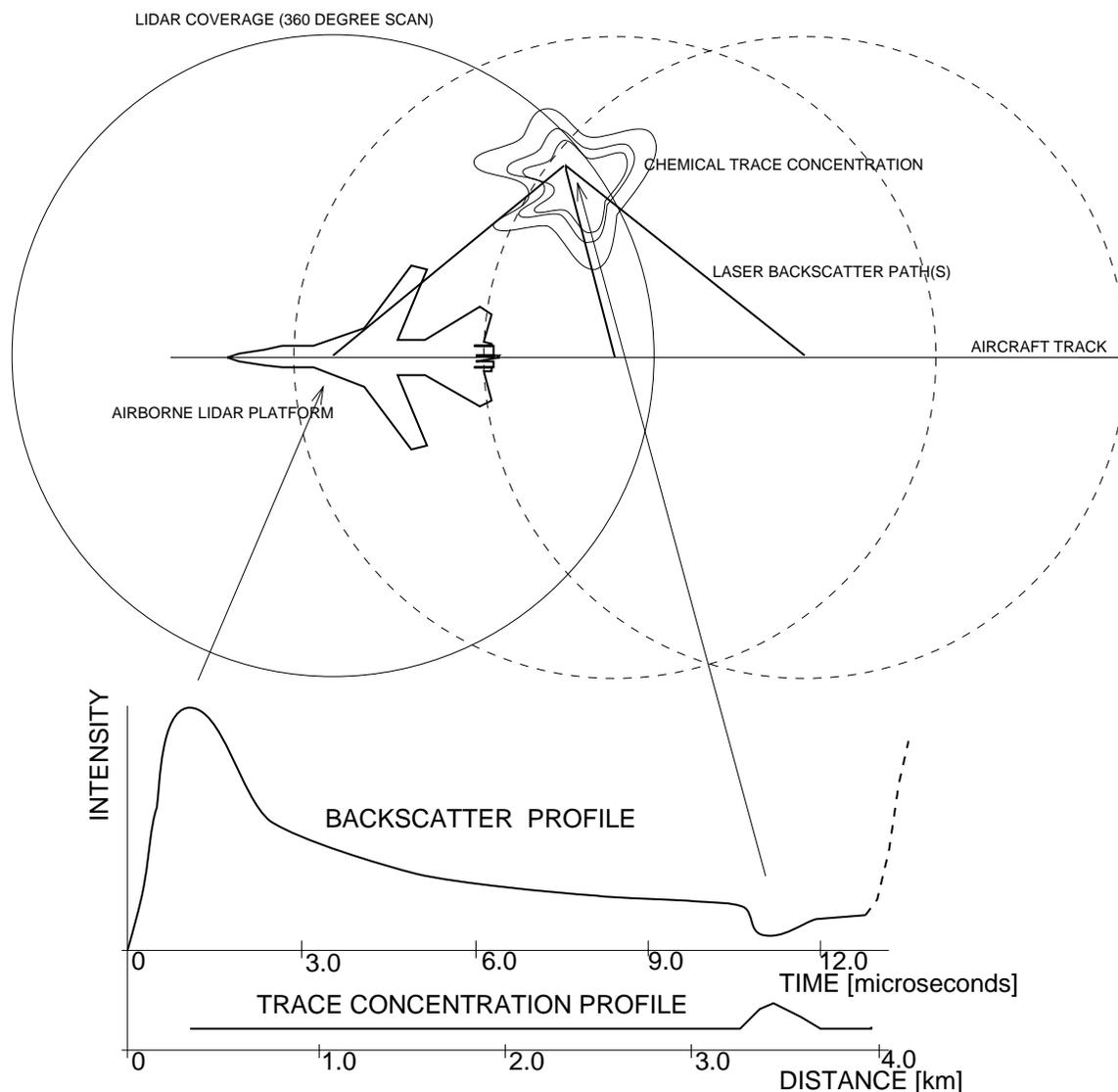
**FIG 6. CIRCULAR SCAN PATTERN AIRBORNE LIDAR ARRANGEMENT - RECCE**
