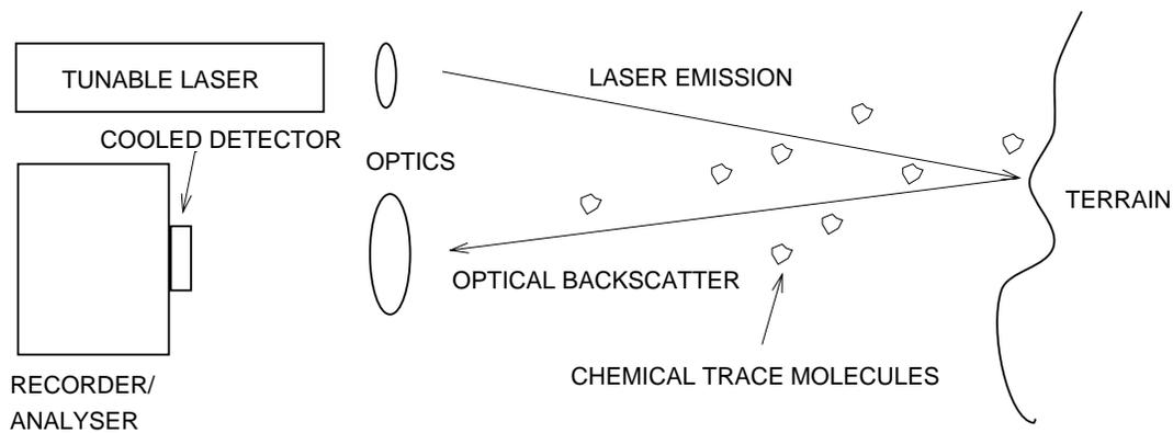
FIG.3.1 SIMPLIFIED SCHEMATIC OF AN LIDAR (ABSORPTION) SPECTROMETER
