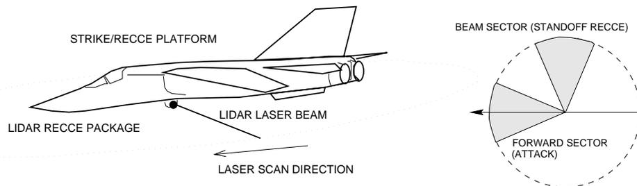
**FIG 7.2. CIRCULAR (PPI) SCAN PATTERN AIRBORNE LIDAR ARRANGEMENT**
