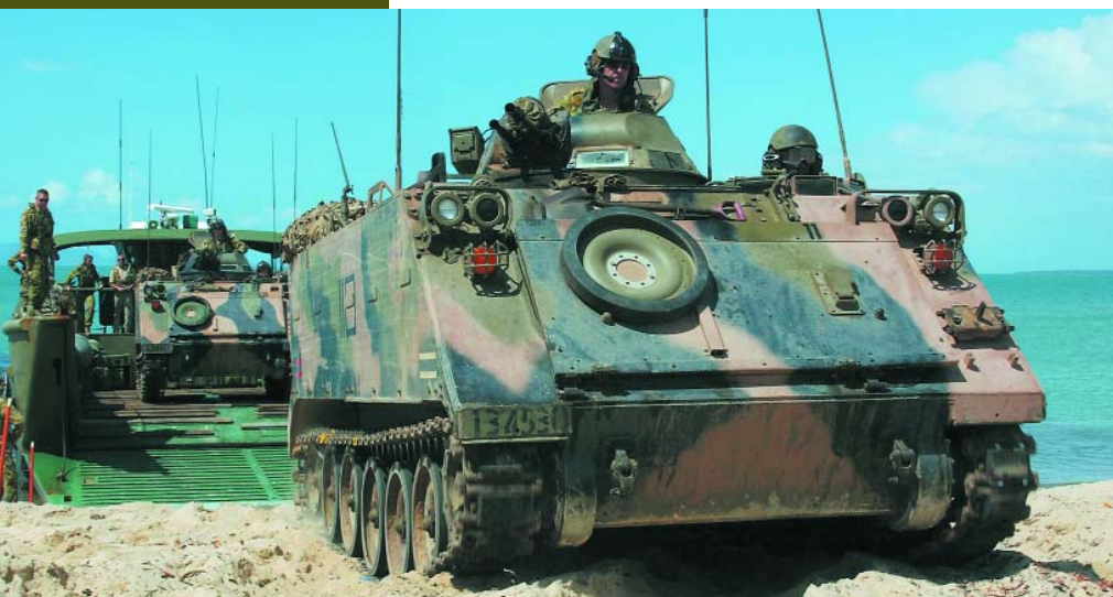
M113A1 armoured personnel carriers unload during an exercise in Shoalwater Bay. Tenix is currently modifying M113A1s into the M113AS3 and AS4 configurations, the latter a hull stretch not unlike the US M113A4 MTVL and Canadian MAV.
