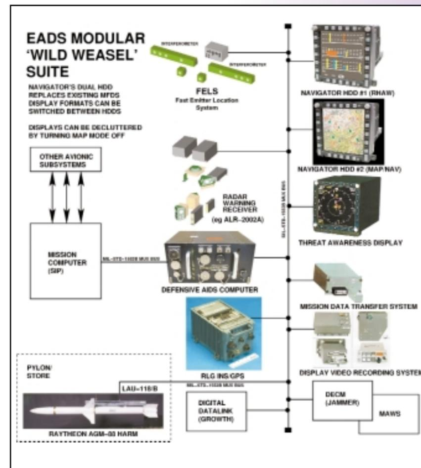
The strength of the EADS proposal lies in the fully autonomous 360-degree coverage of an improved Tornado ECR system - superior to the in-service Tornado ECR package. The aircraft can perform reconnaissance and SEAD independent of standoff electronic surveillance platforms, providing a fully self-contained package.
