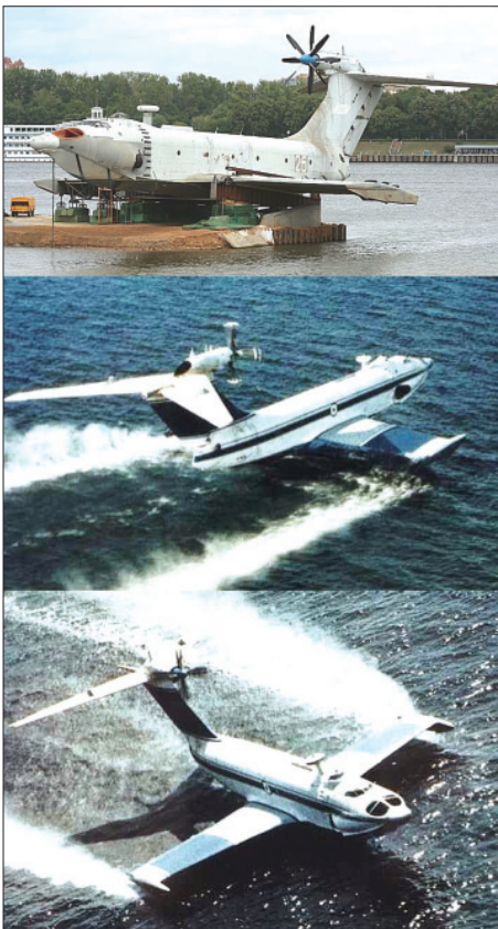
The 30 tonne payload class A.90 Orlyonek Ekranoplan was specifically designed for amphibious assault operations. The whole nose hinges to the right, exposing a ramp for RORO vehicle deployment and recovery. The A.90 cruised at 200 KTAS with an 800 NMI range. Only three were used operationally.
