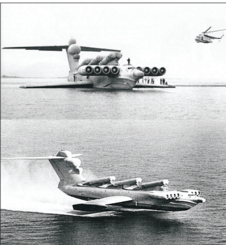
The 400 tonne gross weight Izdelye 903 MD-160 Lun Ekranoplan was developed for a range of roles, the sole demonstrator equipped with six SS-N-22 Sunburn ASCMs. It cruised at nearly 300 KTAS, and had a range of 1,600 NMI.
