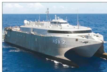
Wave piercing catamarans are a useful technology in logistical support of deployed forces, with high speed and RORO configuration well suited to sealift operations.
