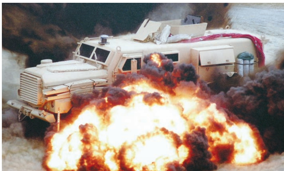
The increasing potency of manportable anti-vehicular weapons such as IEDs and RPGs has effectively rendered the traditional light motorised infantry force model obsolete. This US Marine Corp Cougar MRAP is being tested for blast resistance.
