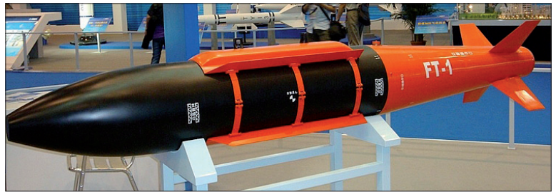
The Luoyang FT-1/FT-2 “Sino-JDAM” are equivalents to the GBU-32 JDAM, the latter including a glide wing kit.
