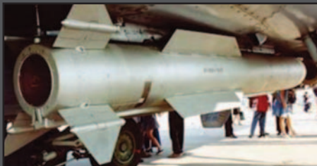
The Vympel R-37 / AA-13 Arrow was the first of the long range counter ISR missiles to emerge. It is equipped with an Agat 9B-1388 active radar seeker, and production variants are expected to be equipped with the new ARG-S-PD seeker.
