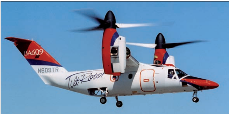
The Agusta/Bell BA.609 is the first tiltrotor design developed for civilian users. It is intended for high revenue markets such as executive transport or oil/gas industry offshore operations.
