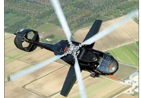
Piasecki / PIAC X-49A Speedhawk or Vectored Thrust Ducted Propeller (VTDP) demonstrator.
