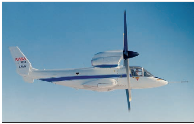
The Bell XV-15 Tiltrotor demonstrator was highly successful, and the basis of the current V-22 Osprey and BA.609.
