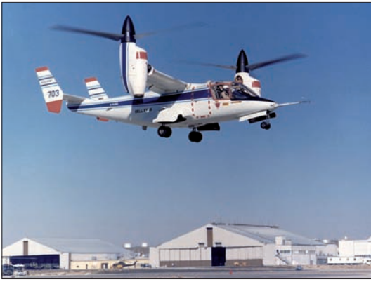
The Bell XV-15 Tiltrotor demonstrator was highly successful, and the basis of the current V-22 Osprey and BA.609.
