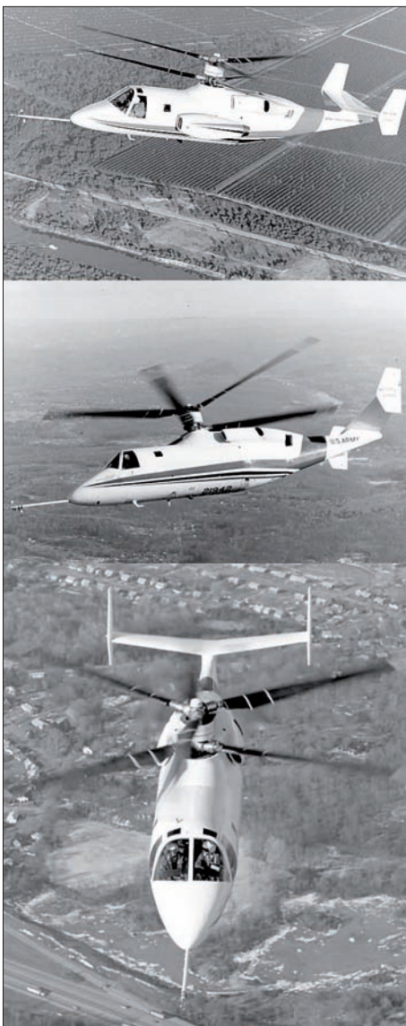
The Sikorsky S-69 / XH-59 Advancing Blade Concept demonstrator was flown for over a decade to prove coaxial rotor and jet propulsor technology. It remains one of the fastest rotary wing designs ever built.
