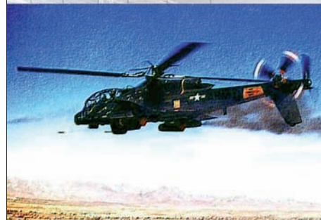
The cancelled Lockheed AH-56 Cheyenne has earned cult status since its cancellation in 1972. It was at that time the fastest combat helicopter design built in the US. It employed a pusher prop as a propulsor, and wing to overcome retreating blade stall, making it a compound helicopter.
