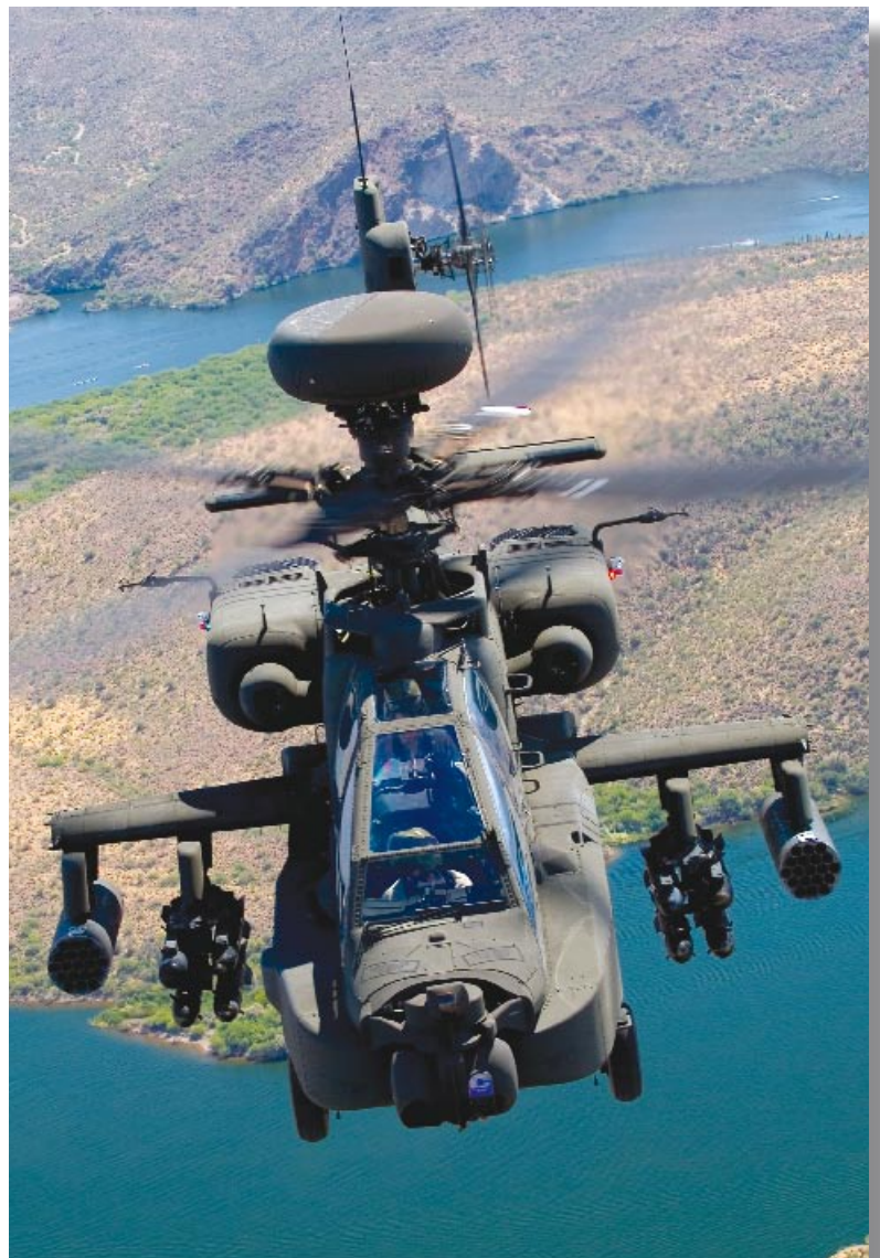
The Longbow radar and MMW Hellfire were developed to defeat the SA-15 Gauntlet and SA-19 battlefield air defence weapons.
