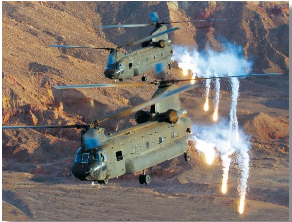
Flares are effective against older MANPADS, but ineffective against newer seeker technologies, and radar directed SAMs and SPAAGs.
