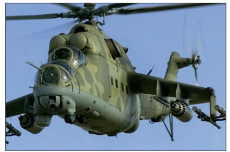
While variants of the UH-1 Iroquois were the first operational gunships, they were soon supplanted by the specialised AH-1 Cobra, which in turn set the pattern for later designs like the Mi-24 Hind (right) and AH-64 Apache (below).
