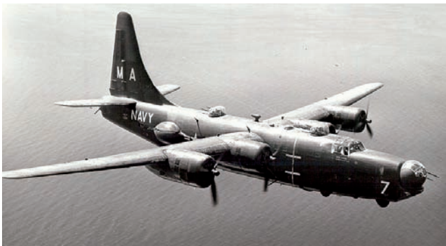
The PB4Y-2 Privateer was the first purpose built LRMP aircraft, deployed in 1944.
