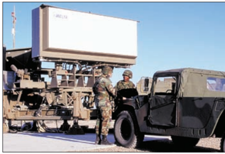
Elta acquisition and tracking radar for the THEL. The radar is used to cue the precision optical tracker on the beam director.
