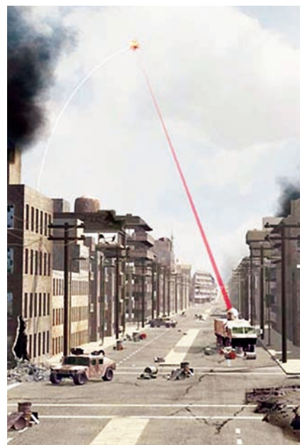
Boeing CONOPS illustration for the HEL TD system, used in the ‘C-RAM’ role against rockets, artillery and mortars.
