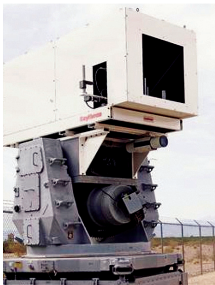
Raytheon's LADS demonstrator uses technology from the Phalanx CIWS and an electrically powered high power optical fibre laser.
