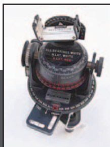
A Mark II Astrocompass, used by navigators in US Army Air Corps bombers such as the B-17, B-24 and B-29.
