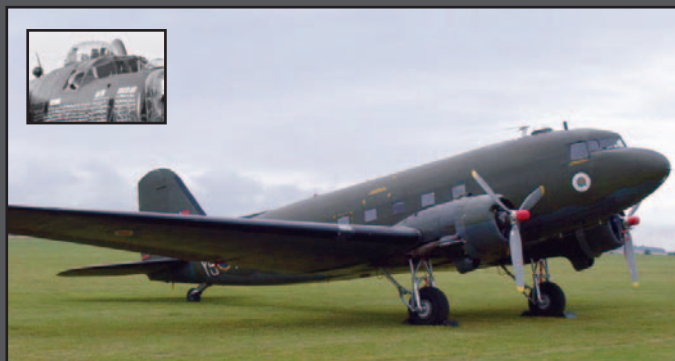
The astrodome was provided so a navigator could take position fixes from stars.
