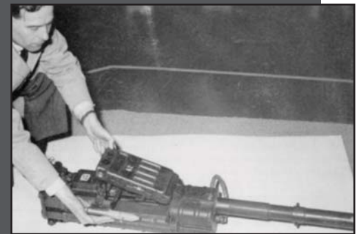
The Lightweight Rheinmetall-Borsig MK 108 was the first 30 mm cannon to be widely used on fighter aircraft, equipping variants of the Bf-109, FW-190, He-219, Me-110, Ju-88, Do-217 and Me-262A. It replaced the much earlier MK 101 design.
