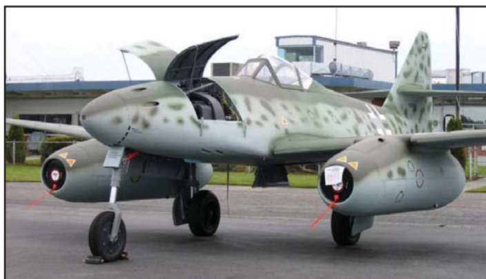
The deadly Me-262A turbojet fighter was armed with four lightweight 30 mm MK 108 guns making it the most heavily armed single seat fighter of WW2. Two exact replicas are being flight tested by the privately funded Me 262 Project in the US. Note the open cannon bay doors (refer Stormbirds.com)
