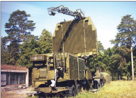
The S-300PMU-1/2 NIIP 64N6E Big Bird phased array best compares in capabilities to the naval SPY-1 Aegis system. This highly mobile search radar can deploy and stow in under five minutes.
