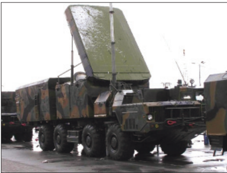
The 30N6E Flap Lid engagement radar is a Russian analogue to the Patriot MPQ-53, but is larger. It is available in high mobility and semi-mobile mast mounted variants.
