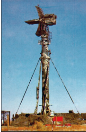
The Clam Shell is a specialised low altitude search and acquisition radar, developed to hunt cruise missiles. It is usually deployed on a semimobile 40V6M or 40V6MD mast system to markedly improve low level coverage.
