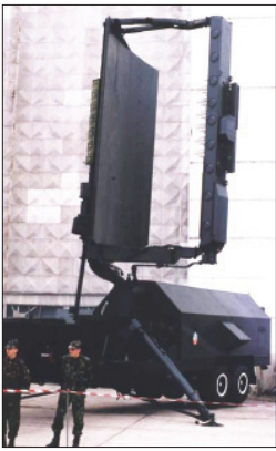
The Clam Shell is a specialised low altitude search and acquisition radar, developed to hunt cruise missiles. It is usually deployed on a semimobile 40V6M or 40V6MD mast system to markedly improve low level coverage.
