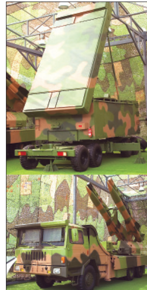
China's indigenous HQ-12 / KS-1A best compares in capabilities to the US RIM-66 SM-1/SM-2 Standard SAMs. The H-200 phased array engagement radar is available in semi-mobile configuration (depicted) or a fully mobile arrangement resembling the Russian 30N6.
