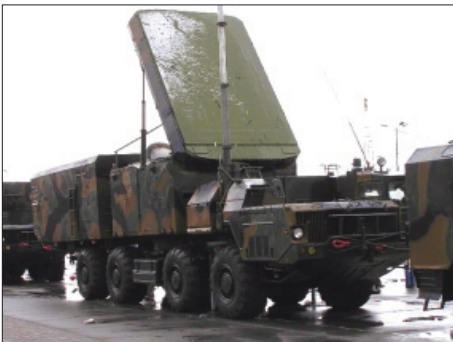
The 30N6E Flap Lid engagement radar is a Russian analogue to the Patriot MPQ-53, but is larger. It is available in high mobility and semi-mobile mast mounted variants.
