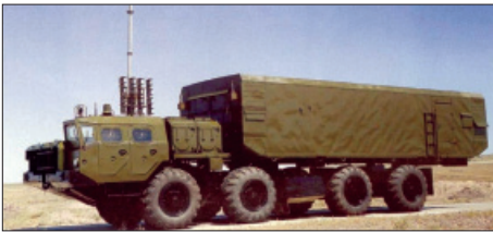
Variants of the 54K6E mobile command post are used with all later variants of the S-300PMU and S-400 systems.
