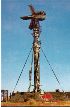
The Clam Shell is a specialised low altitude search and acquisition radar, developed to hunt cruise missiles. It is usually deployed on a semimobile 40V6M or 40V6MD mast system to markedly improve low level coverage.
