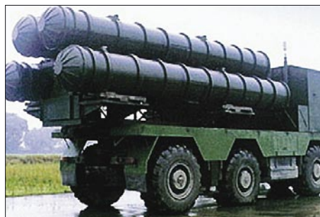
The FT-2000 is a counter-ISR SAM, based on the HQ-9/FD-2000, itself derived from the Russian S-300PMU series.
