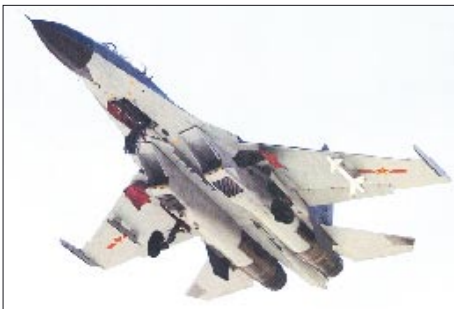
The J-11B is a sophisticated derivative of the Su-27SK rather than a clone, with internal systems much closer to current built Russian Flankers.
