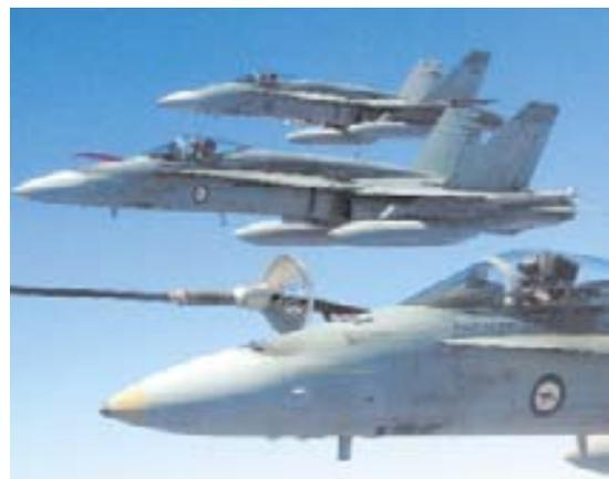
The F/A-18A recently received the APG-73 radar, AMRAAM and ASRAAM missiles, an IFF interrogator and new computers and displays under the HUG program. The plan for early retirement of the F-111 sees a full Mil-Std-1760C capability added to the F/A-18A and the AIR 5418 Follow-On Stand Off Weapon and AIR 5409 GPS aided bombs integrated.
