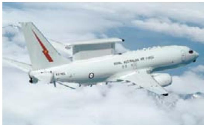
*The jewel in the crown of the RAAF's ISR capabilities will be the new Wedgetail AEW&C aircraft, to be flown by a reconstituted 2 SQN. The Wedgetail is the most advanced AEW&C aircraft developed to date, using the new L-band MESA phased array.*
