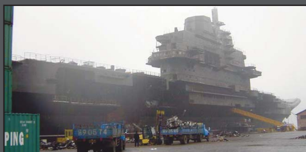
After many years in limbo, China has moved the former Soviet carrier Varyag to a drydock for a major refit. At 67,000 tonnes this carrier is designed to embark Su-33 and Su-27KUB navalised Flankers.
