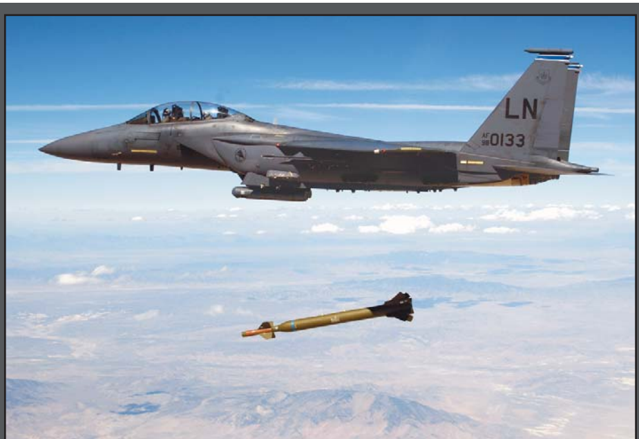
South Korea's F-15K is the most advanced production variant of the F-15E to date. It incorporates all of the incremental upgrades developed for US F-15C and F-15E aircraft, in addition to F110 engines and SLAM-ER/Harpoon capability (USAF).
