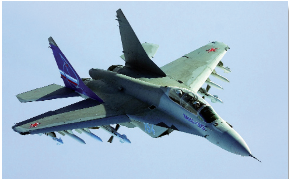
The MiG-35 radar, technologically comparable to the Super Hornet's APG-79 AESA, is a hot favourite in the Indian MRCA contest, and is the first Russian fighter with an active phased array (AESA) radar (top).
