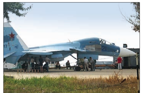
Su-33UB demonstrator equipped with TVC engines and Zhuk MSFE PESA radar.
