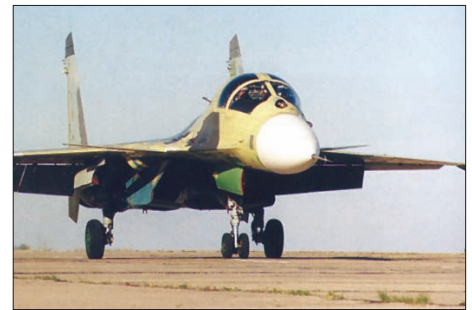
Prototype Su-27KUB showing the side by side cockpit.
