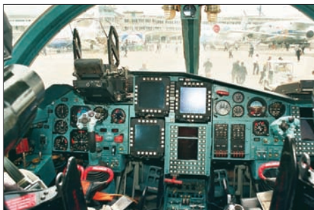
Su-34 demonstrator cockpit. LRIP aircraft are expected to have a new arrangement with AMLCD displays.
