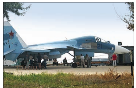
Su-33UB demonstrator equipped with TVC engines and Zhuk MSFE PESA radar.
