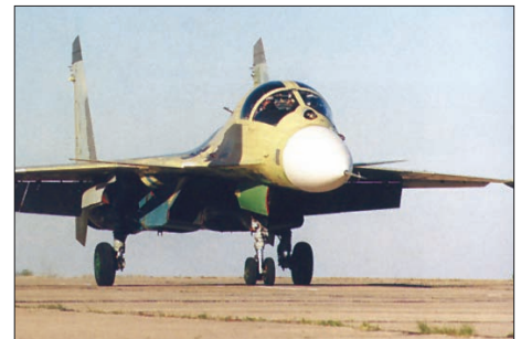
Prototype Su-27KUB showing the side by side cockpit.
