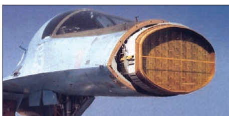
The Leniñets B004 PESA attack radar is conceptually similar to the B-1B's APQ-164.
