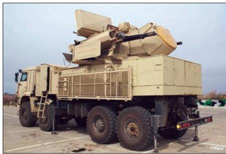
*Like the SA-15D, the Pantsir S1 / SA-22 Greyhound is tasked with killing smart munitions, it is equipped with phased array acquisition and engagement radars.*
