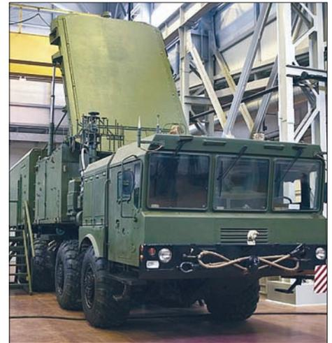
*The S-400's 92N2E Grave Stone engagement radar is a digital design. It is a growth derivative of the 30N6E series, equivalent to the US MPQ-65 radar.*
