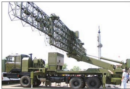
The entirely new Vostok E two metre band is claimed to acquire an F-117A at 190 nautical miles. It can stow and deploy using an elevating and telescoping mast in a mere 8 minutes. With such mobility it directly competes against current and legacy L-band, S-band and X-band SAM system radars.
