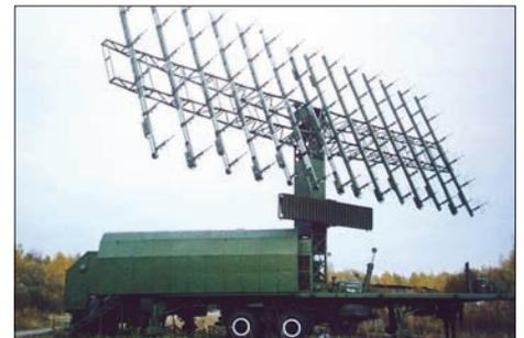
The Nebo SVU is the first ever VHF band AESA. Its agile electronic beamsteering provides it with similar tracking capabilities to the US SPY-1 Aegis series, but operating in the two metre rather than S-band.
