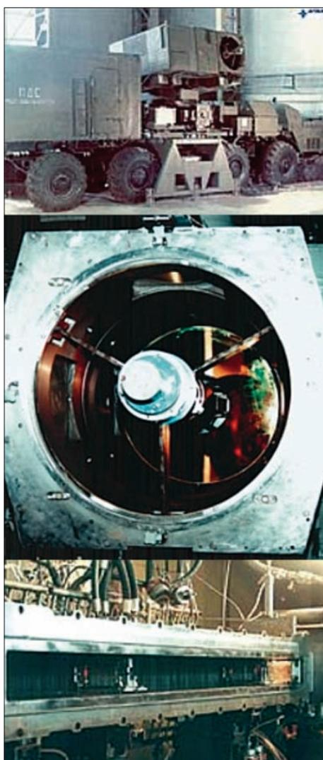
The Almaz-Antey high energy laser weapon demonstrator uses a gasdynamic (chemical) laser. It is technologically similar to the US THEL/MTHEL weapon. While Russian industry has maintained a low profile in laser weapons, China has a large research and development program in high power chemical and free electron lasers, and adaptive optics, intended to defeat PGMs and cruise missiles.
