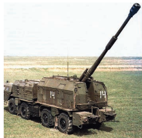
The A222 Bereg 130 mm SP Gun is a Russian built coastal defence system, carried on a modified MAZ 543 8x8 chassis. There are no known SPH variants.
