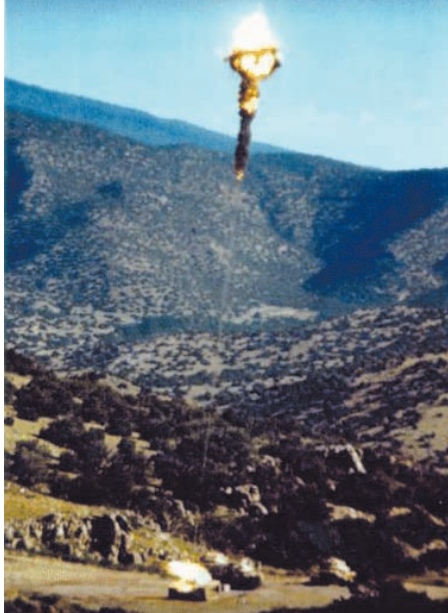
The M898 SADARM (Sense and Destroy Armor) is a smart submunition which uses a combination of infrared scanning and millimetric wave radar to detect targets and initiate its charge, which creates a high velocity slug for top armour attack (US Army).
