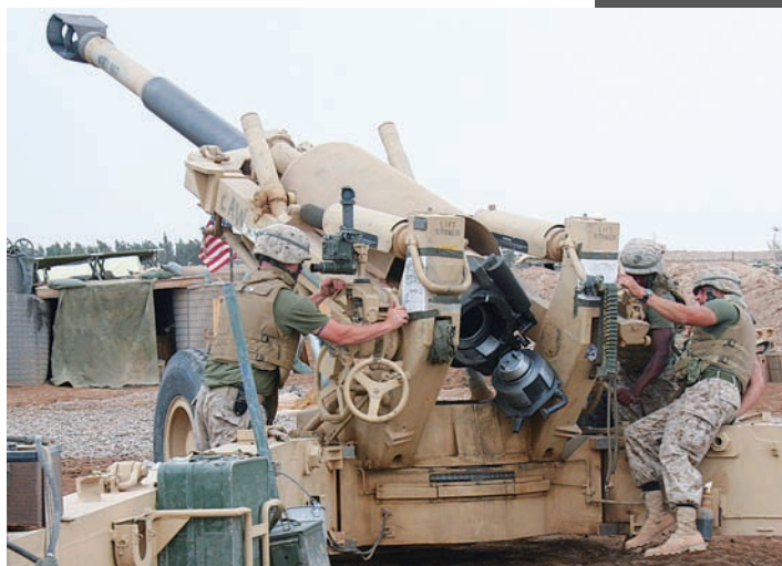
US Marines at Falluja prepare an M198 155 mm towed howitzer for firing. The M198 is the largest artillery piece used by the Australian Army (USMC).
