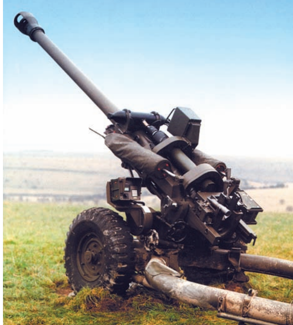
The L119 Hamel gun is used primarily to support infantry. It is a light 105 mm weapon, which can be towed or slung beneath a helicopter (BAe).
