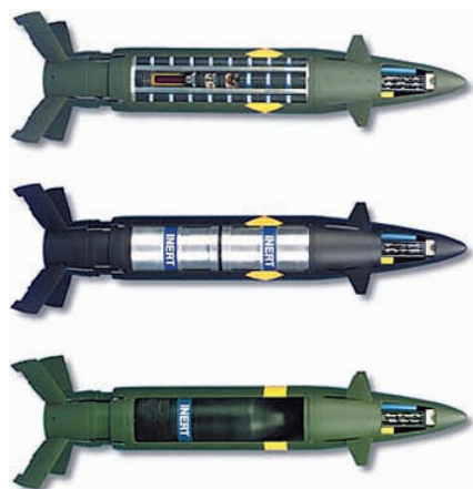
The M982 Excalibur Precision Guided Extended Range Artillery Projectile is a 155 mm GPS/inertial guided munition with base bleed range extension, and the choice of DPICM dumb bomblet submunitions, SADARM smart submunitions, or a unitary warhead (US Army).
