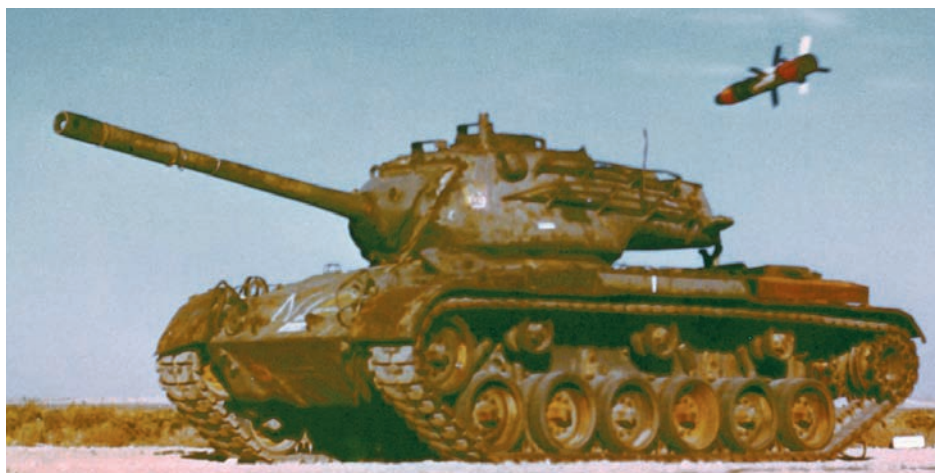
The M712 Copperhead was the first semi-active laser homing artillery munition to enter production, designed primarily as a precision guided anti-tank munition (US Army).
