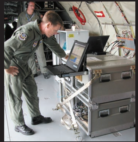
The ROBE demonstrator system during trials performed at Eglin AFB in 2002. The system integrates a laptop computer running gateway software, a MIDS/LVT network terminal and an ARC-210 UHF satcom radio (US Air Force).
