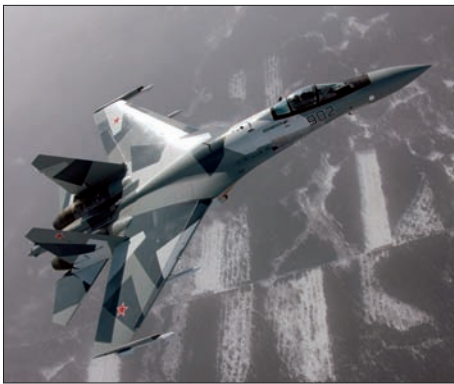
While the Su-35S visually resembles earlier Flanker variants, the redesign is deep and comprehensive. The new glass cockpit is modelled on the F-35 arrangement but employs mature low risk AMLCD technology.
