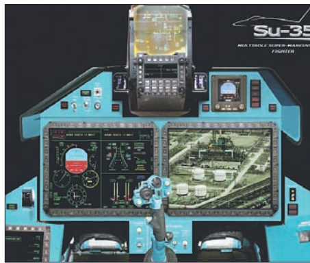
While the Su-35S visually resembles earlier Flanker variants, the redesign is deep and comprehensive. The new glass cockpit is modelled on the F-35 arrangement but employs mature low risk AMLCD technology.
