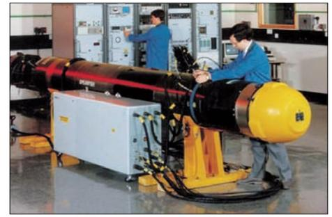
*The Marconi (BAe) Spearfish uses Otto fuel to power a gas turbine, which drives the pumpjet.*
