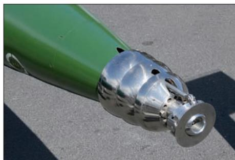
The supercavitating GNPP Shkval is the fastest torpedo in operational use at this time, capable of exceeding 200 knots. The gas generator in the nose produces a supercavitation bubble using the nose mounted exhaust port. The booster solid rocket exhausts through a circular array of nozzles, the sustainer solid rocket exhausts through the central nozzle. The technology has been acquired by China and Iran.
