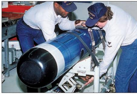
*The Alliant-Techsystems Mk.50 Barracuda or Advanced Lightweight Torpedo torpedo uses an unusual propulsion scheme, where steam is generated using a chemical heat source, to drive a pump-jet.*
