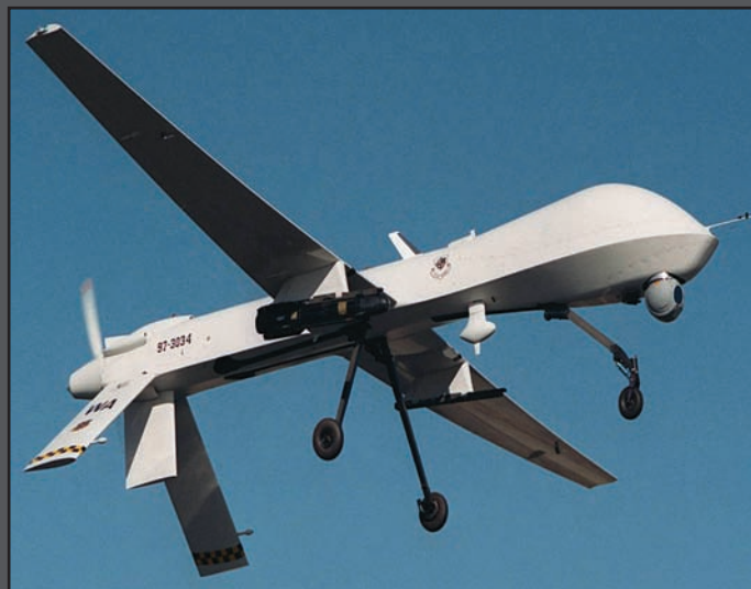
An MQ-1 Predator armed with an AGM-114 Hellfire missile. Predator's primary mission is interdiction and conducting armed reconnaissance against critical, perishable targets. (USAF)
