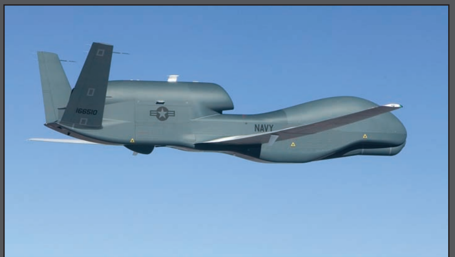
RQ-4B Global Hawk is a much larger, faster, longer ranging and higher flying jet powered airframe, explicitly designed to replace the legacy manned U-2.
