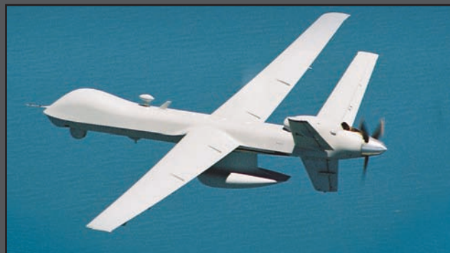
The General Atomics offering for BAMS is the 'Mariner', which is a derivative of the Predator B airframe, with the extended wing designed for the ALTAIR remote sensing UAV and a mission specific payload.
