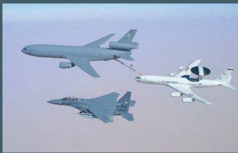
Aerial refuelling is vital to extending the on-station endurance of AEW&C aircraft. (US Air Force)
