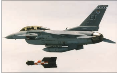
The US Air Force EDGE High Gear program trialled an extremely accurate Wide Area Differential GPS scheme for weapons guidance. Depicted images from drops of modified GBU-15 glidebombs, using only differential GPS guidance.
