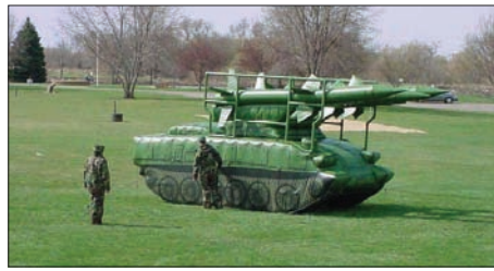
right: Corruption attacks deceive the opponent as to the identity of a target. Decoys are an excellent example of seductive corruption attacks. Depicted inflatable decoys made by Aerostar Inc.
