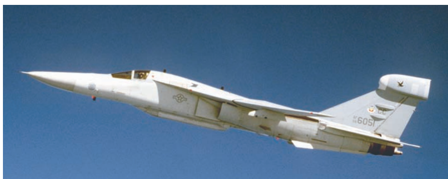
Noise jamming of radar is an active degradation attack. Depicted are Cold War era EF-111A Raven and Spoon Rest D.
