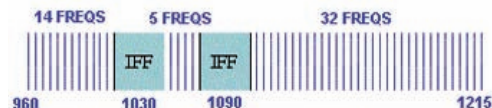
JTIDS Frequencies. JTIDS hops between a total of 51 separate frequencies (US Navy).
