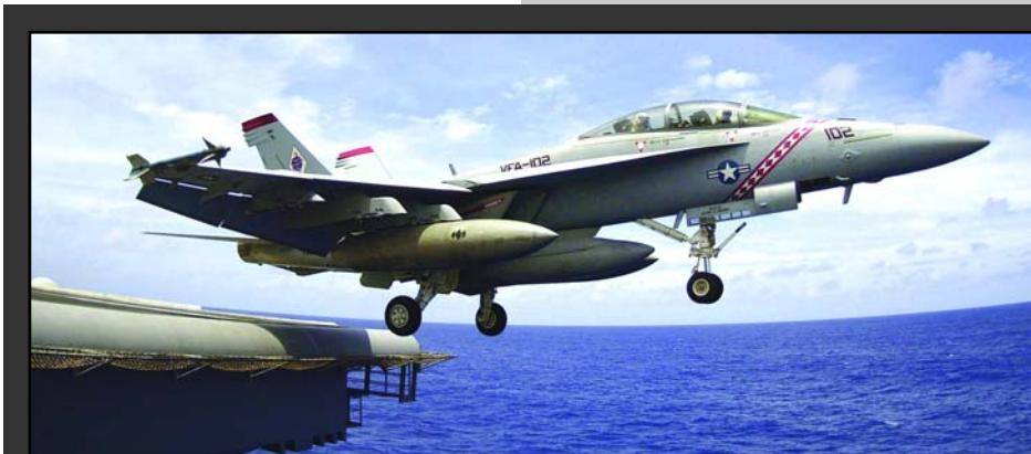
An F/A-18F Super Hornet launches from the flight deck of the USS Kitty Hawk equipped with a Shared Reconnaissance Pod (SHARP), a multi-functioned reconnaissance pod used on the F/A-18F Super Hornet for tactical manned airborne reconnaissance. (Jonathan Chandler, US Navy)
