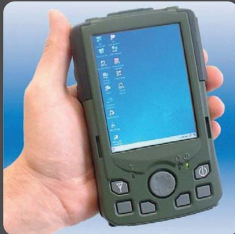
With a choice of Win PC 2003 or Win CE, and a range of inbuilt and add-on options including GPRS, CDMA, GPS, Radio ID scanners, barcode scanners, wireless and hard-wired LAN adapters, long-life batteries, docking stations and GSM phone, this really is the go-just-about-anywhere, do-just-about-anything Rugged PDA you've been looking for!
