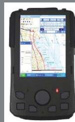
With a choice of IP54 (rated to survive 4" of rain per hour) or IP67 (rated to survive to 1m underwater for 30 minutes) and with a full Type II PCMCIA slot, plus an SD card slot, plus dual in-built antennae, the 'Openfire' RPDA lets you move previously desk-bound applications out into the field for increased productivity.
