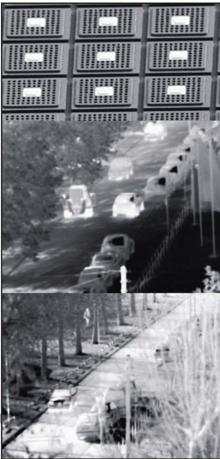
Top: a nine pixel closeup of a QWIP imaging chip, the small dots are the actual quantum well structures.
