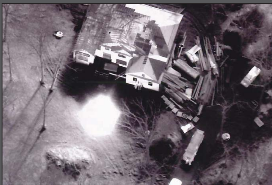
Imagery produced by L-3 Cincinnati Electronics 2048 x 2048 pixel midwave band imaging array (L-3).
