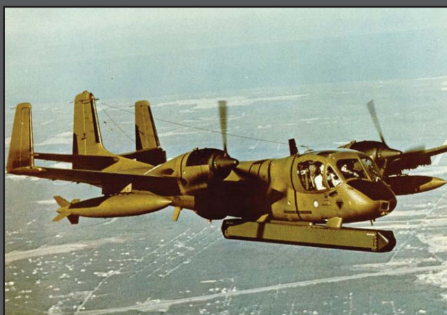
OV-10 equipped with the massive APS-94 SLAR, an example of a high resolution real beam mapping radar. Note the sheer size of the sidelooking antenna.
