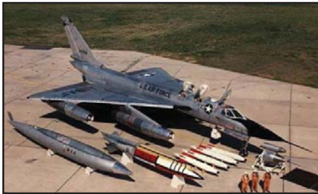
The first SAR used operationally was carried over Cuba by a B-58 Hustler, the radar being carried in a special ventral pod.
