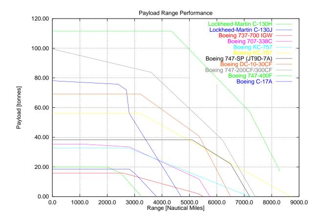
Figure 16: Comparison of payload/radius performance for representative aerial refuelling aircraft (Author, Boeing and other data).
