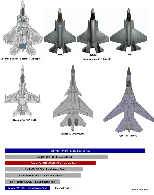
RELATIVE COMPARISON OF SIZE AND INTERNAL FUEL CAPACITY Provisional Data
