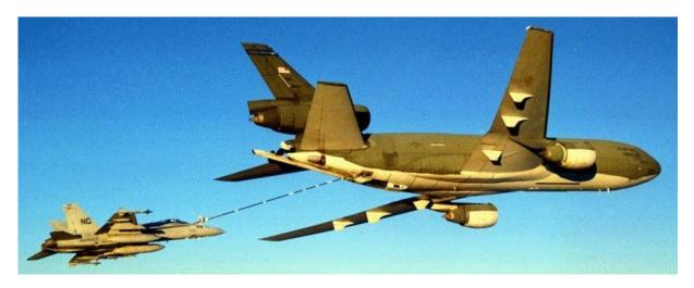
Figure 10: The Boeing (MDC) KC-10A is based on the DC-10-30CF airframe, which was superceded by the MD-11. With the recent completion of MD-11 production, the supportability of the US Air Force's 59 strong KC-10A fleet will be compromised once most of the commercial DC-10-30 fleet is retired in the 2010-2015 period, if not earlier due to the airline industry collapse (US Air Force).
