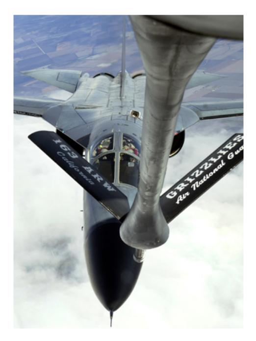
Figure 7: The RAAF's F-111C/G aircraft employ the US Air Force standard boom refuelling system, unlike the F/A-18A which uses the US Navy/RAF standard hose/drogue refuelling system. Coalition operations with allies might involve refuelling aircraft using either system, therefore the RAAF's new tankers must have facilities for both. The existing Boeing 707-338C tankers are not equipped with booms (RAAF).
