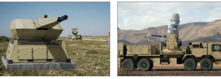
Modern Counter Rocket Artillery Mortar (C-RAM) systems can be readily adapted for the Counter PGM roles, but will require significantly better engagement radars, capable of tracking, sorting and engaging multiple inbound high speed PGMs. Depicted a Luftwaffe MANTIS/Skyshield 35 mm gun system, and a prototype high mobility Phalanx C-RAM system on a modified Oshkosh HEMMT chassis.
