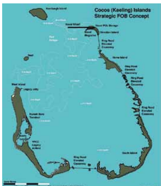
Concept diagram for Cocos Islands redevelopment. This and similar basing arrangements are viable for high tempo combat operations, while providing peacetime eco-tourism potential. Environmental impact is minimised by siting the airfield on the unused coconut plantation, and placing the wharf outside the central lagoon (Author).
