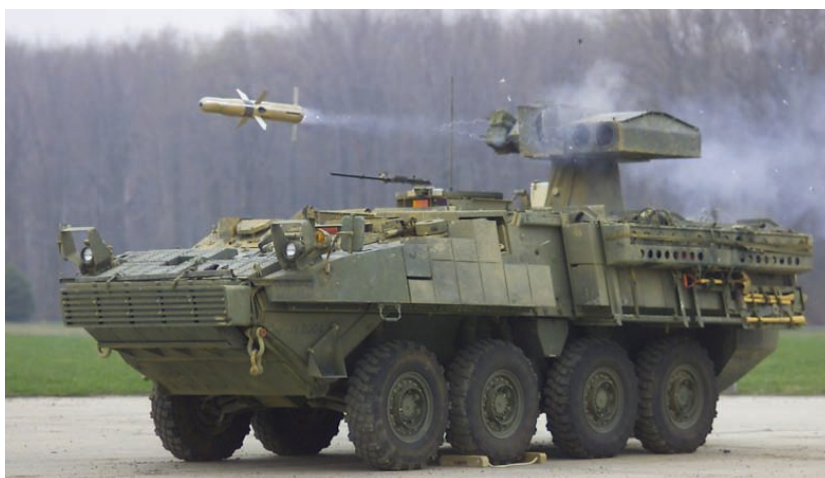
M1134 Stryker Anti-Tank Guided Missile. The ATGM variant is intended to provide a highly mobile anti-tank capability, using a remote control turret with sensors and a pair of TOW missile launcher tubes. The system is intended to supplement the MGS.
