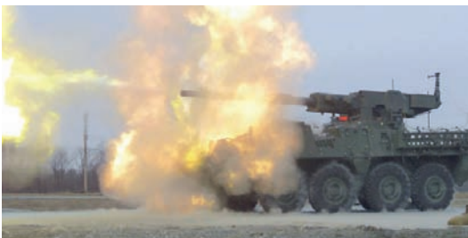
M1128 Stryker Mobile Gun System. The Stryker brigades will derive much of their fire power from the MGS system, which is equipped with a 105mm gun common to early variants of the M1 Abrams tank. The MGS has a stabilised turret, permitting the three-man crew to fire on the move.
