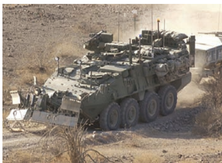
M1132 Stryker Engineer Support Vehicle. The ESV is intended to support mine clearing and obstacle removal tasks.
