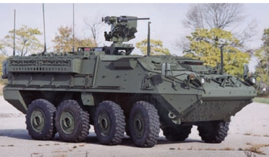
M1126 Stryker Infantry Carrier Vehicle (LAV-III). The core of the BCT Striker brigades is the ICV, which has a crew of two and carries nine infantrymen .
