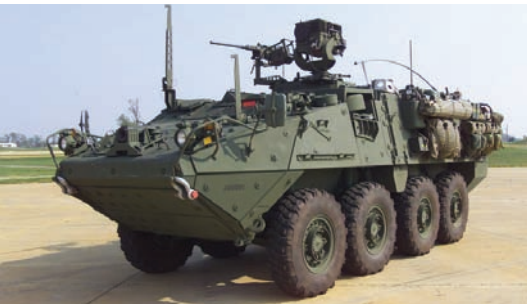
M1127 Stryker Reconnaissance Vehicle. The RV is intended as a platform for deploying six strong scout teams. The baseline vehicle is also common to the M1129 Stryker Mortar Carrier, equipped with a 120 mm and 60 mm mortar for indirect fire roles.
