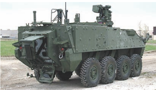
M1135 Stryker NBC Recon Vehicle. The NBC RV is intended to perform nuclear, biological and chemical reconnaissance in contaminated terrain. It includes full NBC capability including an overpressure system.
