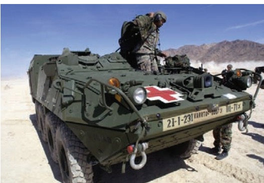
M1135 Stryker NBC Recon Vehicle. The NBC RV is intended to perform nuclear, biological and chemical reconnaissance in contaminated terrain. It includes full NBC capability including an overpressure system.
