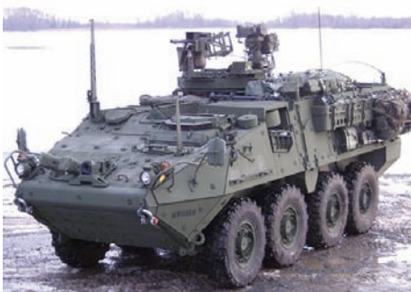
M1131 Stryker Fire Support Vehicle. The FSV is a sensor platform with a laser ranging / designation capability, and a communications package, intended to facilitate direct and indirect fire support.
