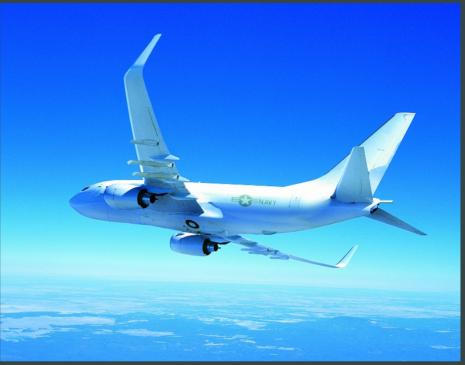
The Boeing MMA is based on the 737-800 airframe, but uses the heavier -900 series wing.
