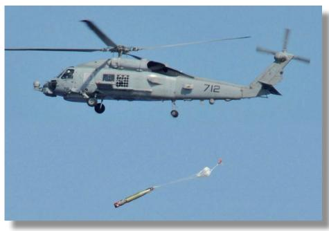
Drop of a Mk-46 lightweight ASW torpedo from a Seahawk ASW helicopter.
