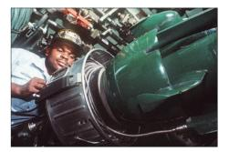
The Mk-48 ADVCAP is a heavyweight torpedo powered by an Otto fuel gas generator driving a shrouded propulsor. A cable tether is used to transmit midcourse guidance commands.
