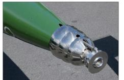
The supercavitating GNPP Shkval is the fastest torpedo in operational use at this time, capable of exceeding 200 knots. The gas generator in the nose produces a supercavitation bubble using the nose mounted exhaust port. The booster solid rocket exhausts through a circular array of nozzles, the sustainer solid rocket exhausts through the central nozzle. The technology has been acquired by China and Iran.
