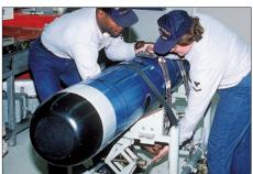
The Alliant-Techsystems Mk.50 Barracuda or Advanced Lightweight Torpedo torpedo uses an unusual propulsion scheme, where steam is generated using a chemical heat source, to drive a pump-jet.
