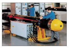
The Marconi (BAe) Spearfish uses Otto fuel to power a gas turbine, which drives the pumpjet.
